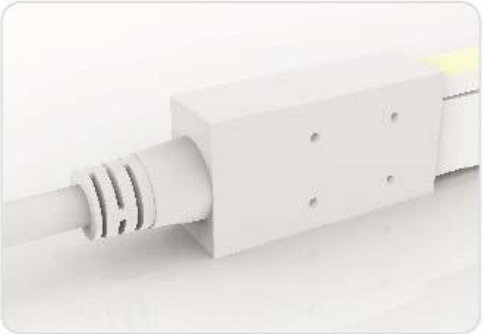
Double Injection Moulded Side Entry—IP68, Factory Fitted Only
